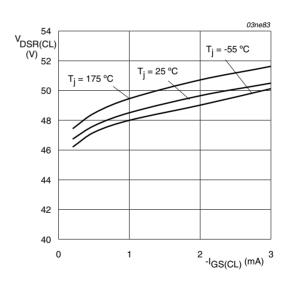
Fig 16. Drain-source clamping voltage as a function of gate current; typical values
