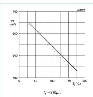
Fig 17. Forward voltage of temperature sense diode as a function of junction temperature; typical values
