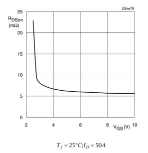
Fig 6. Drain-source on-state resistance as a function of gate-source volatage; typical values
