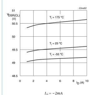
Fig 15. Drain-source clamping voltage as a function of drain current; typical values
